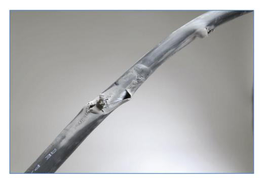
Figure 2. Heat-shrink tubing can be used to repair worn and damaged wire and cable.
