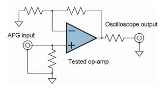
Figure 1: Slew rate measuring circuit.
