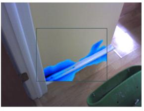
Like with roof leaks, thermal cameras can be used to find moisture trapped in walls and floors. Damp areas change temperature more slowly than dry areas, and are subject to evaporative cooling. This slow change in temperature allows them to become visible to the thermal camera. Causes of this unwanted moisture include plumbing leaks, leaks from the outside, and condensation.
