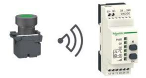
Utilizing wireless technology, the Harmony XB5R wireless, batteryless push button is easy to install in both new and existing applications, such as bottling, packaging and conveying lines. Now, you no longer need to pass a cable through the machine structure or cable tray to connect the push button to the electrical panel – cutting installation costs by 20% as compared to traditional wired solutions.
